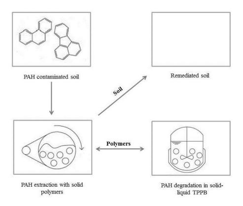
**Fig. 2.** The process of removal of contaminated soil with PAH, treatment process includes PAH recycling from the soil followed by its removal from biphasic system [20].
