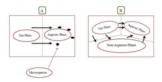
Fig. 1. Difference of mass transfer in biphasic and monophasic systems [8].
